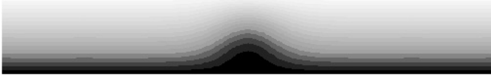
Figure 6: The temperature field generated by the initial perturbation in the 192 \times 32 finite element grid. This is the first frame in every trial run regardless of rheological law, physical parameters, or the Rayleigh number.
